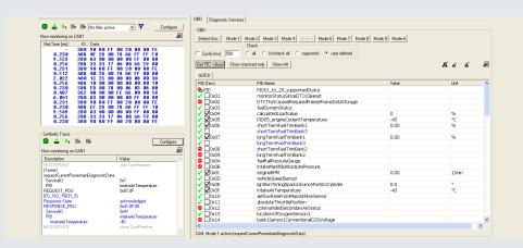
DTS OBD is a PC-based tool for validating and releasing the self-diagnosis of individual ECUs or an entire vehicle in vehicle engineering. It covers the entire scope of onboard diagnostics and combines the functionalities of an OBD scan tool with those of a data and bus monitor in a single tool.
