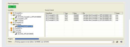
DTS Flash is an easy-to-use tool based on the ODX standard for flash programming of ECUs. It is possible to program one or more flash sessions of an ECU.
