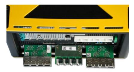
12 Ethernet ports implemented on 3 individual add-on modules enable various Ethernet and Automotive Ethernet combinations. Each module supports either 4 ports in data logging mode or 2 TAP ports; each configurable as PTP/gPTP master or slave. Additional 2 10 GbE ports enable data logging and TAP of multiplexed sensory data from popular automotive AI platforms and drive computers.
